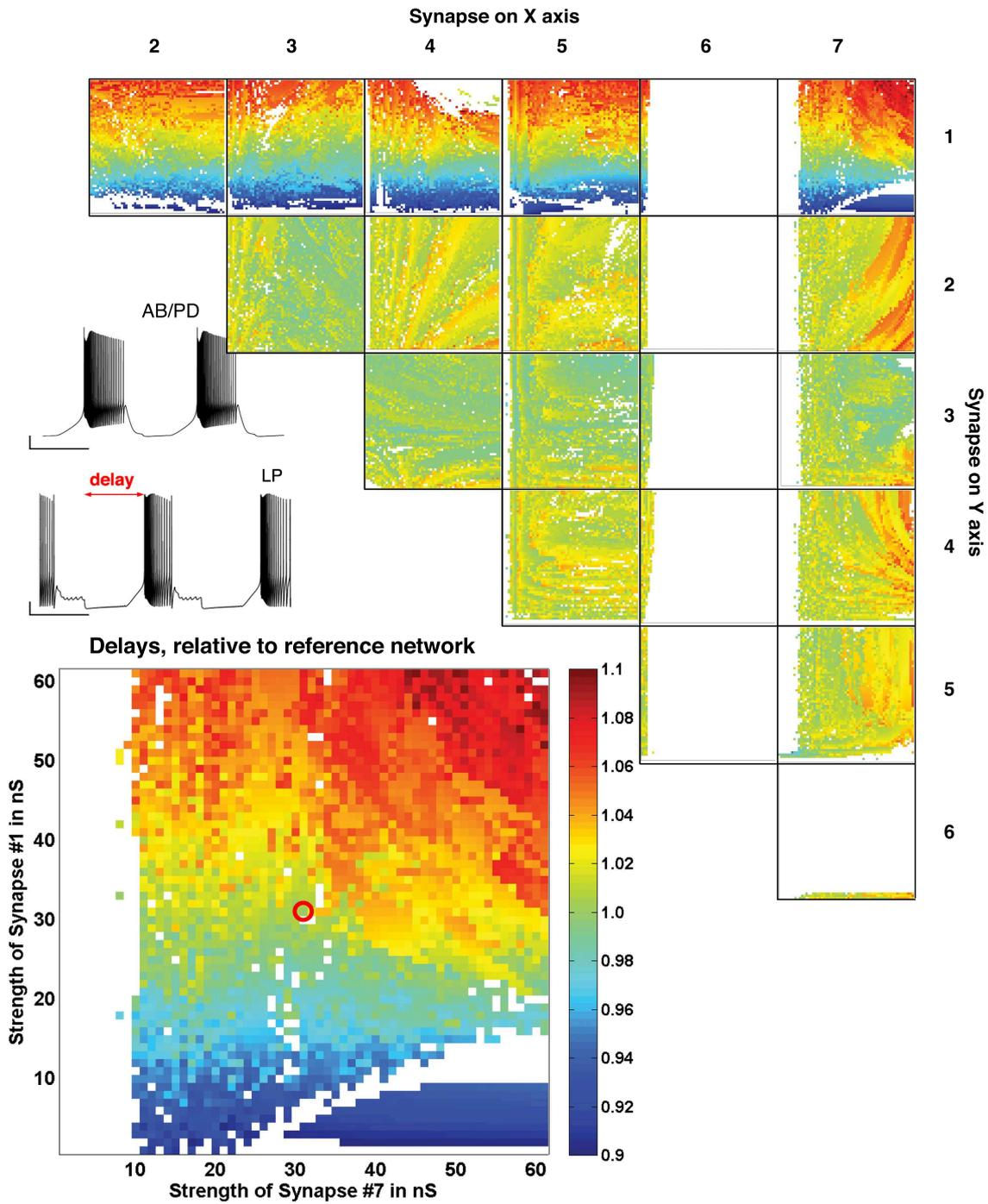
Figure 8: Colour maps of the ratios of delays of 78,141 networks to the delay of the reference network (red circle). All colourmaps as in Figure 5. The magnified colourmap shows dynamical metrics changing smoothly along Synapse # 1, which connects AB/PD to LP. In contrast, the effect of changing Synapse # 7 is more complex, as Synapse # 7 connects PY to LP, leading to more complex network effects.
